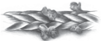
Rope displays two adjacent cut strands -- rope should be replaced.
