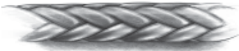
Rope exhibits fiber-set from compression. A slight sheen is visible. This is not a permanent characteristic and can be eliminated by flexing the rope.
